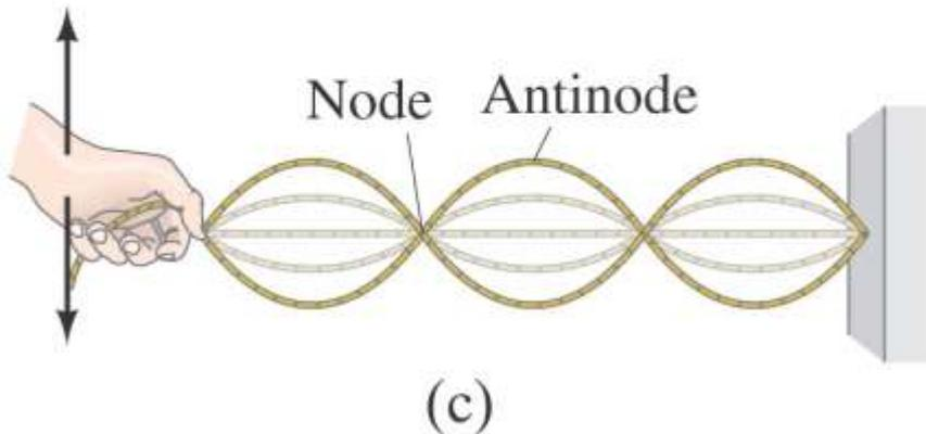
**Standing waves occur when both ends of a string are fixed. In that case, only waves which are motionless at the ends of the string can persist. There are nodes, where the amplitude is always zero, and antinodes, where the amplitude varies from zero to the maximum value.**
