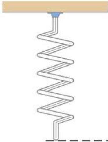
If the spring is hung vertically, the only change is in the equilibrium position, which is at the point where the spring force equals the gravitational force.
