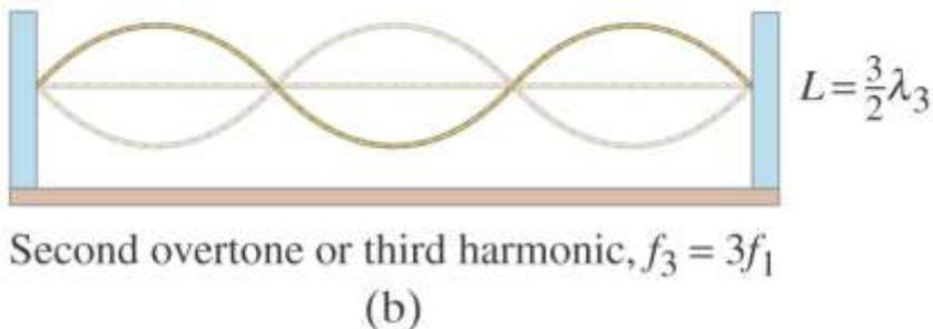
**The frequencies of the standing waves on a particular string are called resonant frequencies.**
