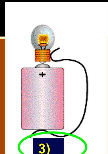
Current can only flow if there is a **continuous connection** from the negative terminal through the bulb to the positive terminal. This is only the case for Fig. (3).
