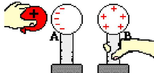
Sphere B is separated from sphere A using the insulating stand. The two spheres have opposite charges.
