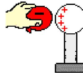
The sphere is now charged positively, with the excess charge attracted to the balloon.
