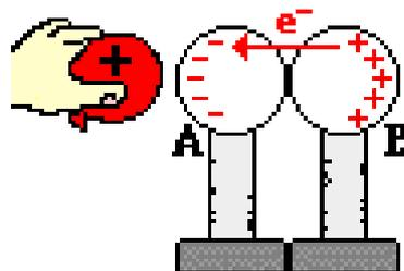
The presence of a + charge induces  $e^-$  to move from spheres B to A. The two-sphere system is polarized.
