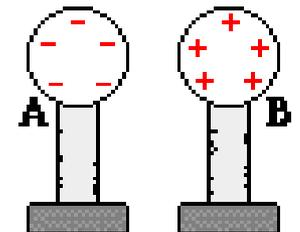
The excess charge distributes itself uniformly over the surface of the spheres.
