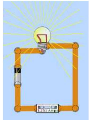
Ammeter configured to measure current.
